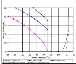
iHA48060A012V-001 maximum output current vs. ambient temperature at nominal input voltage for airflow rates natural convection 0.3 m/s (60lfm) to 3.0m/s (600lfm) with airflow from output to input.
